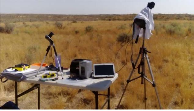
**Figure 1.** Picture showing the equipment employed on 2017 August 21 to acquire the TSE observations analyzed here (see text); the picture shows the DSLR camera mounted on the tripod, connected to remote controllers, and covered by a white tissue to reduce as much as possible the overheating by solar illumination during the PSE.
