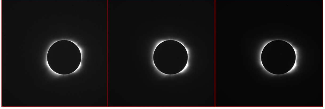
Figure 5.8: Out-band level 0 images at 0^\circ , 60^\circ , 120^\circ [Fineschi et al., 2010a].
