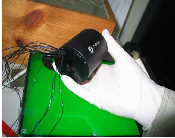
Figure 4.3: The filter prior to adding the electrical connector for LCVR control [Fineschi et al., 2010b].
